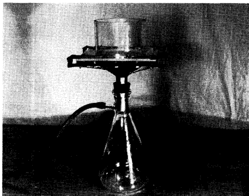
FIG. 2. Holder for molecular filters.
