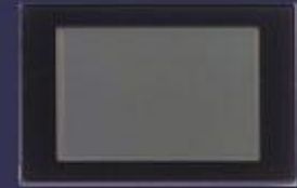
APS-H size sensor: Approx. 29 x 19mm
