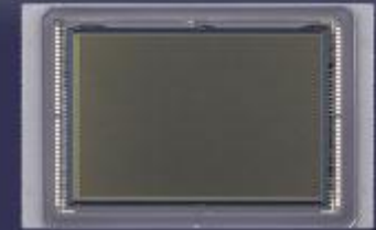
35mm full-frame sensor: Approx. 36 x 24mm
