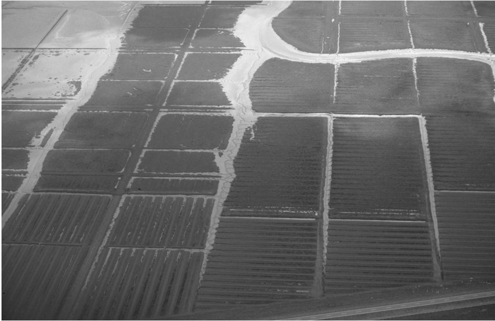
Figure 2. Salt marshes and salt marsh works in the Husum Bight, Schleswig-Holstein (note the regular and intensive drainage pattern in the salt marshes. View from the North).
