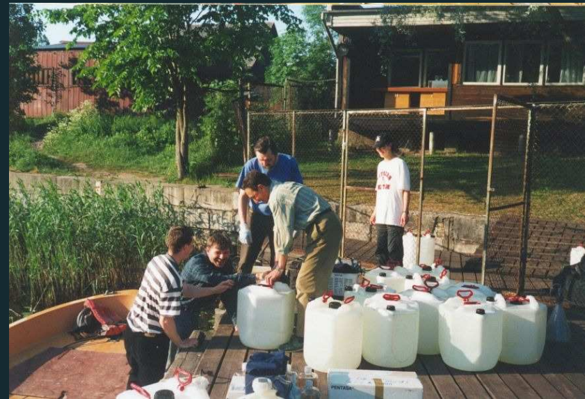
Seawater (400 L) was collected in the upper layer with 8 L Niskin bottles, and after filtration through 150 \mu m mesh, distributed in 50 L carboys
