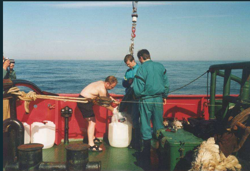
Seawater (400 L) was collected in the upper layer with 8 L Niskin bottles, and after filtration through 150 \mu m mesh, distributed in 50 L carboys
