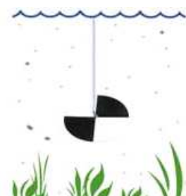
Clear lake having a small algal population results in a deep SDT reading, high clarity
