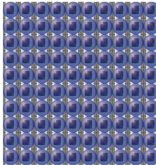
...and put a tiny lens („microlens“) in front of each.
