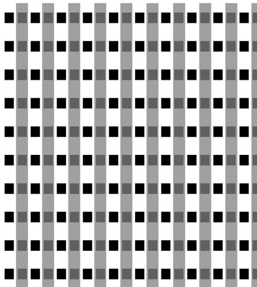
Interline transfer sensors have an integrated electronic shutter called a „dark register“. Pixel charge is transferred to this after exposure waiting to be read from the sensor.
