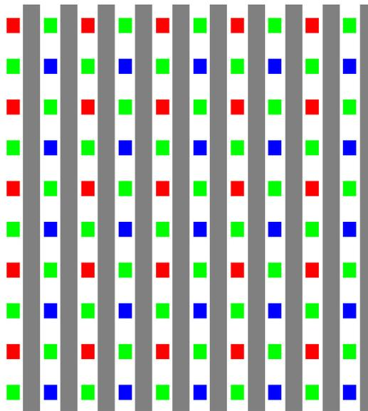
We now could place a small color filter in front of each pixel. But this would leave a large part of the sensor area inactive.
