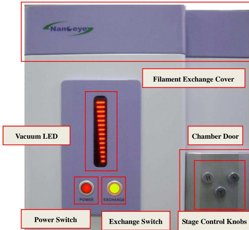
**Fig. 2 Front of Mini-SEM SNE-1500M**
