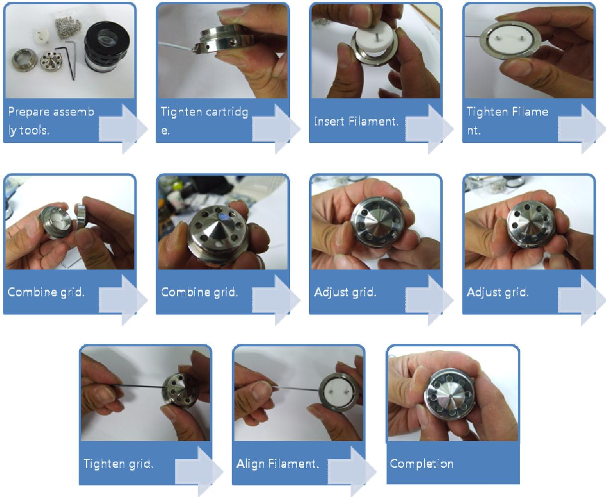
**Fig. 34 Assembly order of Filament and Grid**
