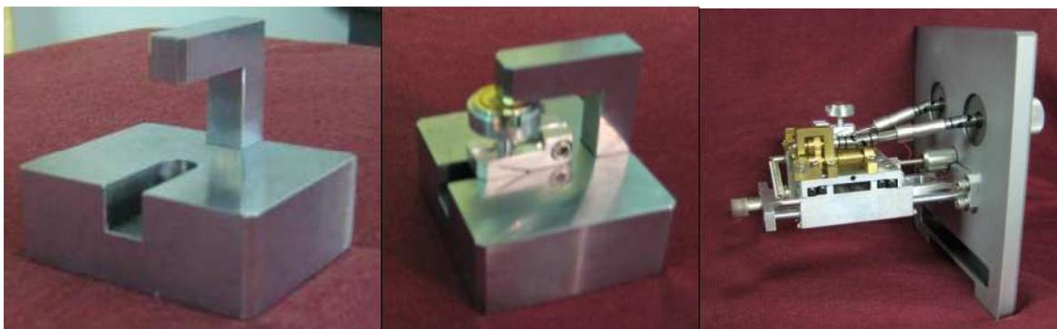
**Fig. 26 Sample Height jig**
