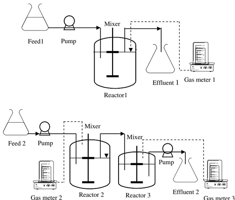
Fig. 1. Lab-scale experimental set-up for one-step (R1) and serial digestion with 70/30 or 50/50% volume distribution (R2 and R3).
