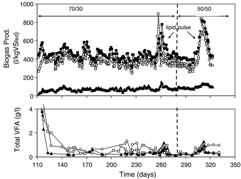
Fig. 3. Process performance and biogas production during anaerobic digestion of cow manure in one-step ((□) R1) and serial digestion with 70/30% and 50/50% volume distribution ((○) R2, (▲) R3 and (■) R2 + R3) in lab-scale at 55 °C.
