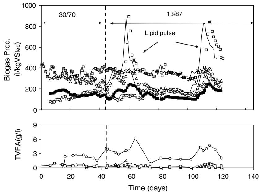
Fig. 4. Process performance and biogas production during lab-scale thermophilic digestion of cow manure in one-step CSTR ((□) R1) and serial digestion processes with 30/70 and 13/87% volume distribution ratios ((○) R4, (Δ) R5 and (■) R4 + R5).
