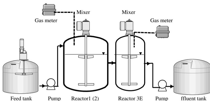
Fig. 2. Pilot-scale experimental set-up for one-step (R1) and serial digestion (R2 and R3) with a volume distribution of 77/23%.
