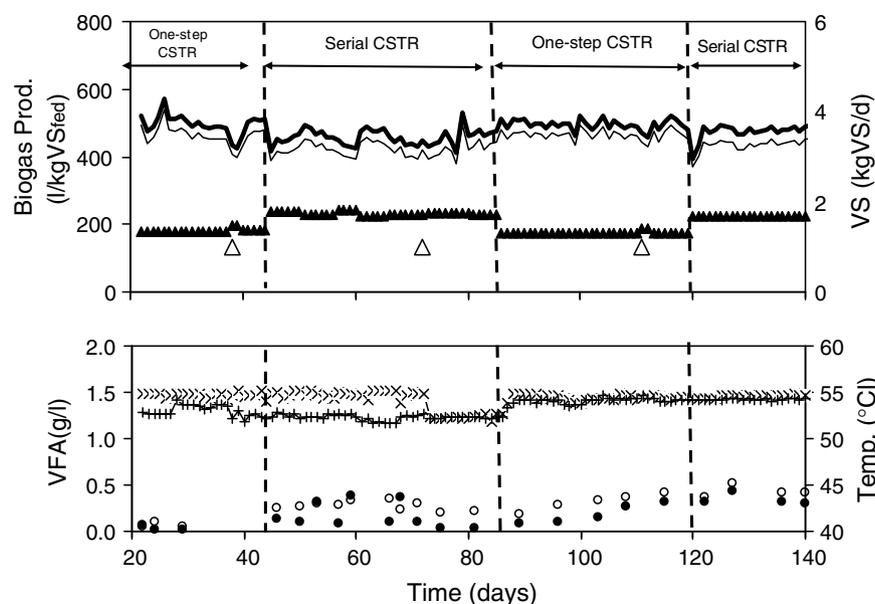
**Fig. 5.** Process performance and biogas production during pilot-scale thermophilic digestion of cow manure in one-step (R1) and serial digestion (R2 + R3) with 77/23 volume distribution: biogas production in R1 (—) and R2 + R3 (—); feed VS ( $\blacktriangle$ ); feed batch changes ( $\Delta$ ); total VFA in R1 ( $\circ$ ) and R2 + R3 ( $\bullet$ ); temperature in R1 ( $\times$ ) and R2 + R3 ( $+$ ).
