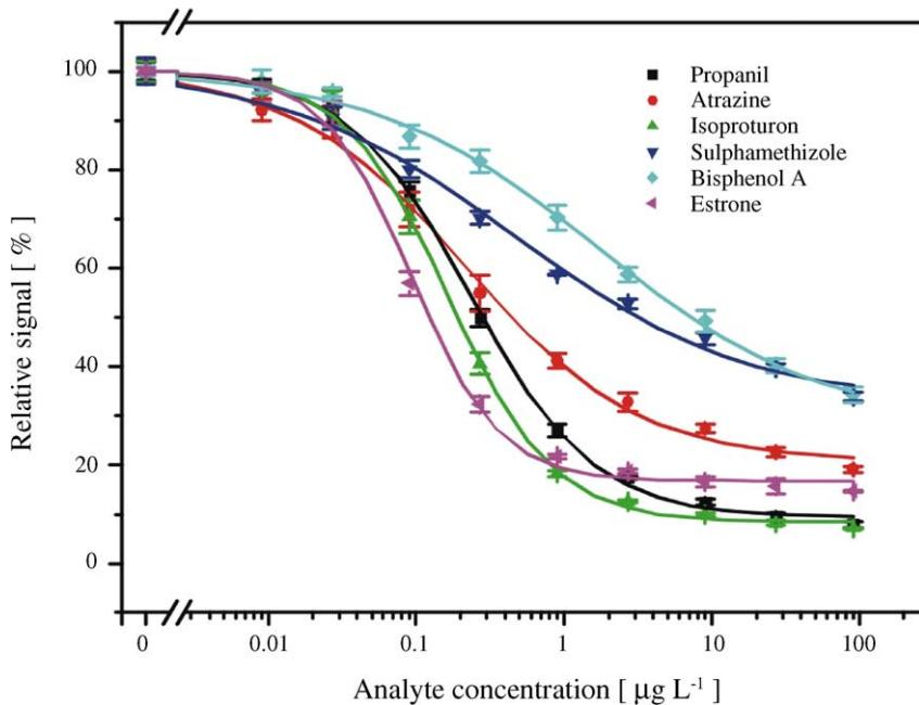
Fig. 3. The resulting set of calibration curves for atrazine, bisphenol A, estrone, isoproturon, sulphamethizole, and propanil which were measured in parallel on a multi-analyte transducer. For all compounds, the calculated LOD is below  $0.020 \mu\text{g L}^{-1}$ .
