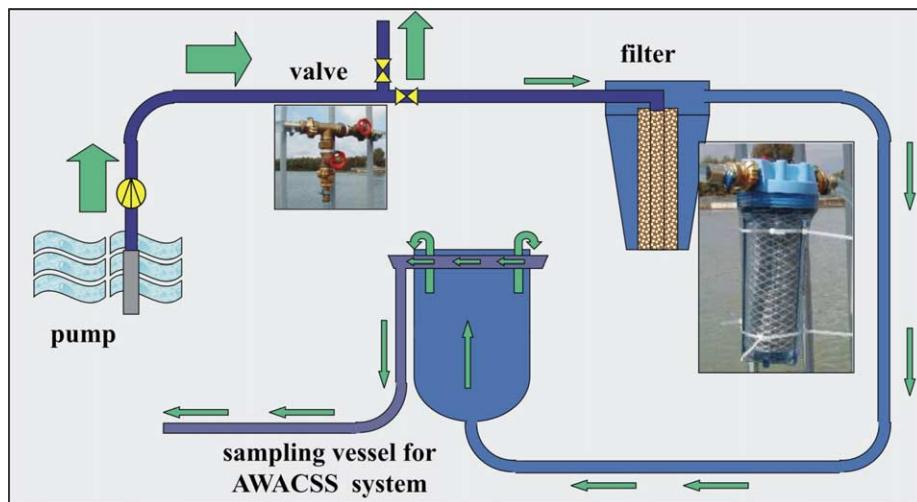
Fig. 1. Schematic set-up of the developed sampling system for on-line monitoring which allows direct intake of river water and its continuous transfer to the autosampler of the AWACSS system.
