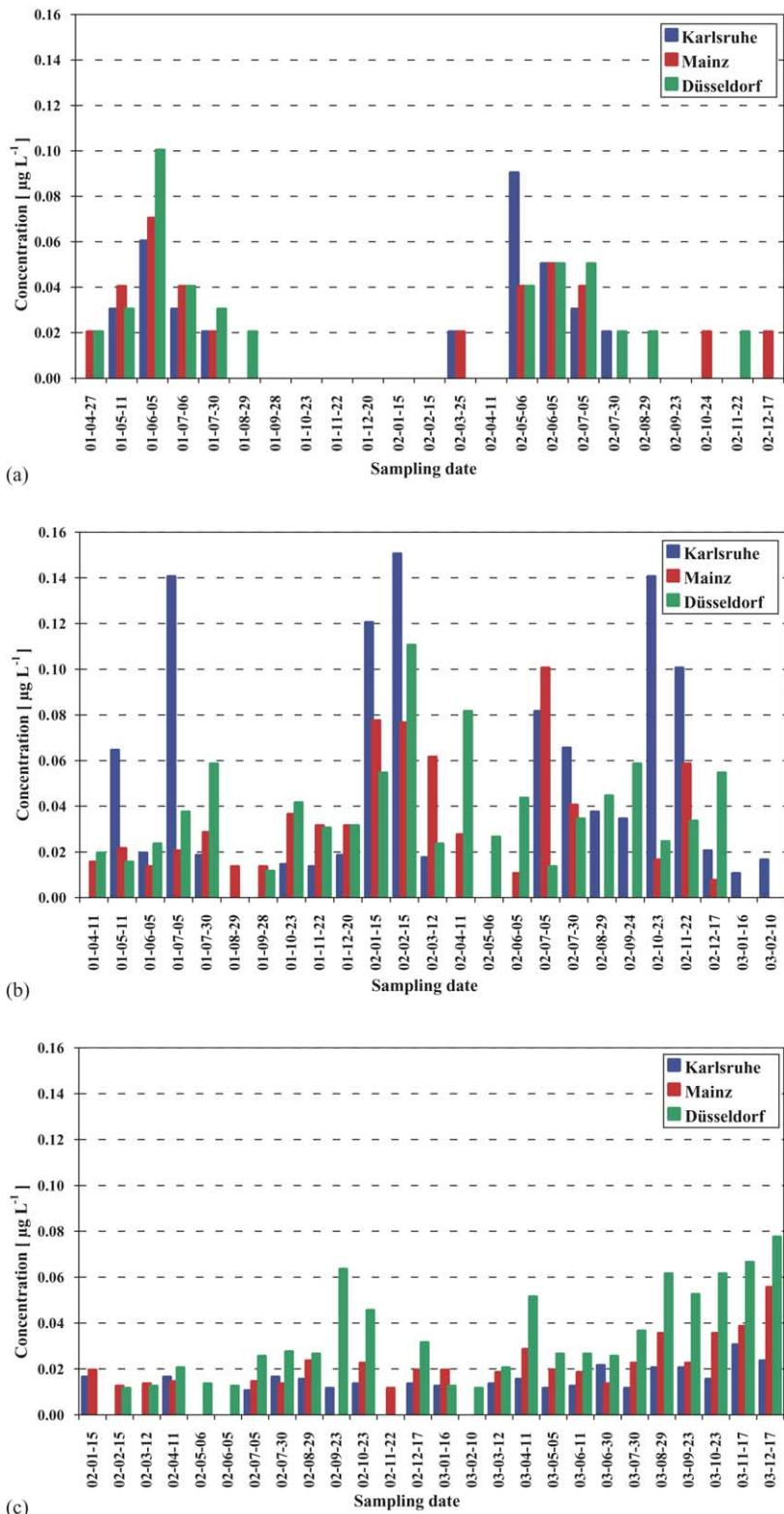
Fig. 2. Characteristic pollution patterns by atrazine (a), bisphenol A (b), and sulphonamethoxazole (c) at the River Rhine (Germany) by GC-MS. Sampling sites: Mainz, Karlsruhe, and Düsseldorf. Results were obtained in the period 2001–2003.
